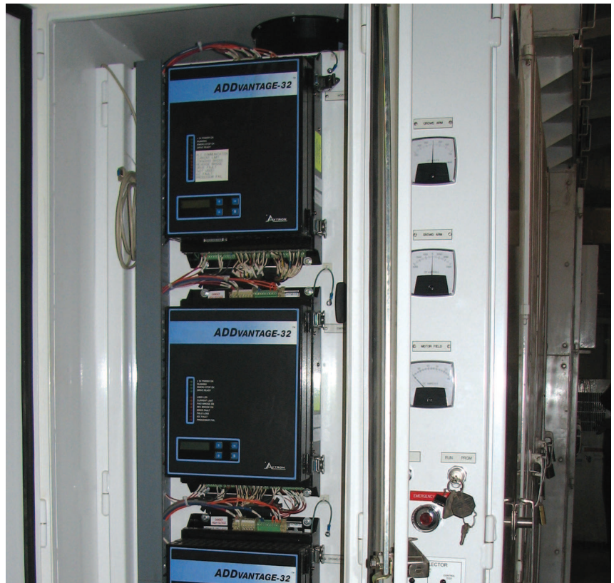
The Power Performance Digital Drive controls the motors to ensure peak power is provided during the digging process.
