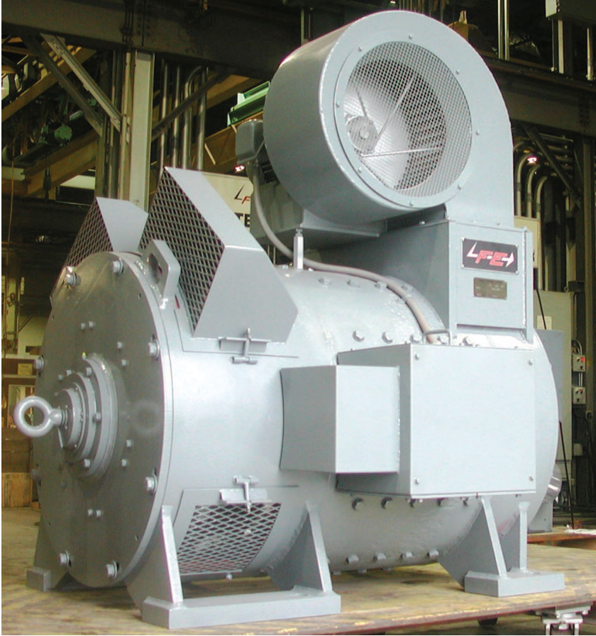
Flanders Electric manufactures motors, such as this hoist motor, specifically for mine-duty applications.
