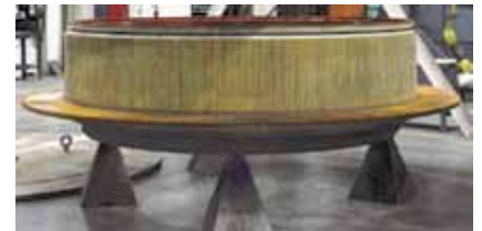
Westinghouse 7000HP commutator insulated and ready to finish turn
