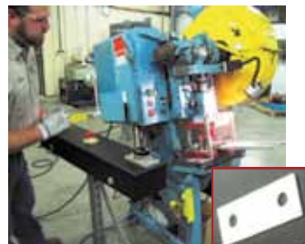
Stamping press produces the finished part (shown in bottom right of photo) for mill motors and generators
