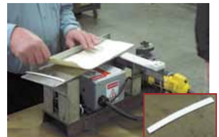
Nibbling cutter cuts armature insulator strips (shown in photo in bottom right) that fits between armature coils
