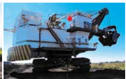
4100A Shovel walking off the erection pad and onto the pit after upgrades
