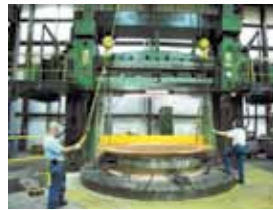
Matt Nussmeier and Matt Kirby setting up to machine the copper assemble prior to assembly onto the installed steel components
