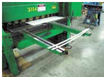
Shear for cutting insulator strips for gang connections for mill motors and generators
